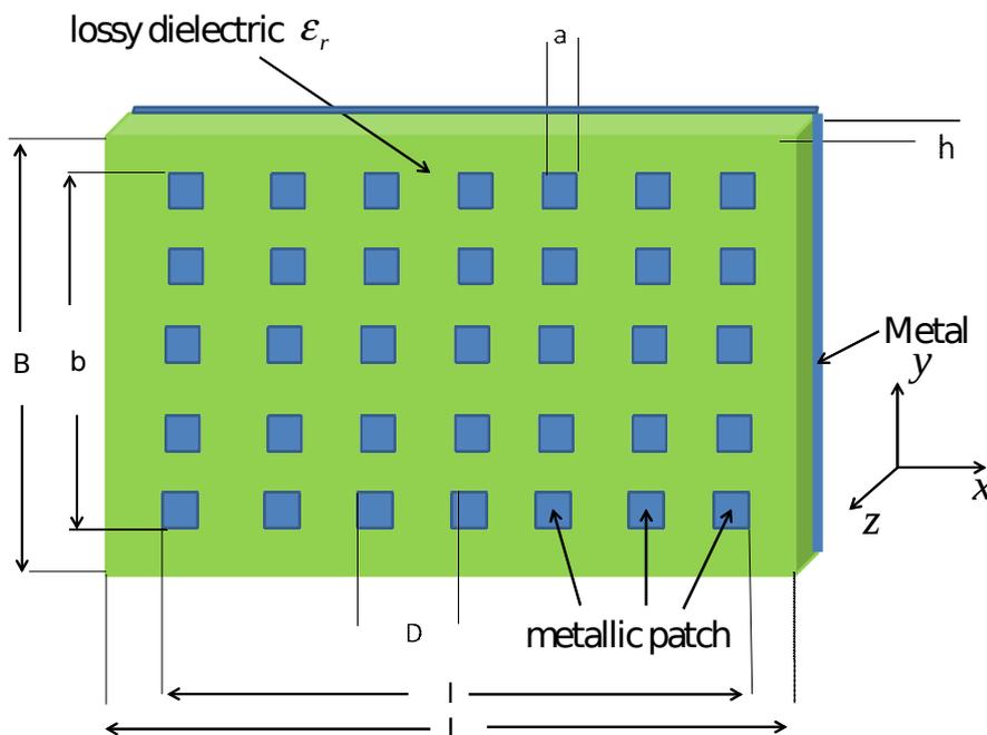
The scattering geometry is represented in the following picture:
