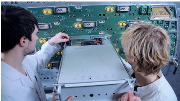
Complex, leading-edge technology in GESTRA: 40 subsystems on 8 enormous circuit boards (130 cm x 55 cm) are mounted directly on the aluminum antenna plate with cooling circuit.
